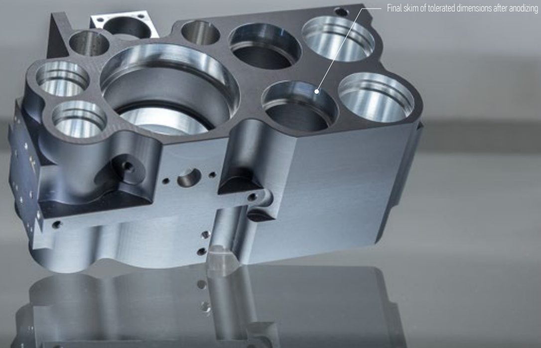
Final skim of tolerated dimensions after anodizing
